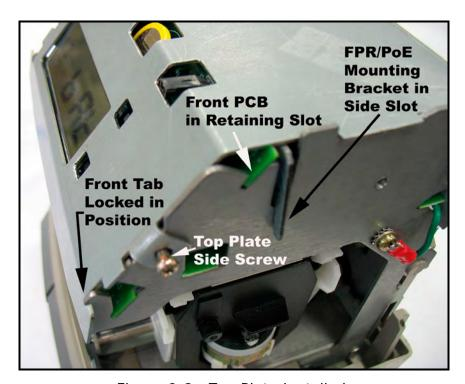
Figure 2-9. Top Plate Installed.
